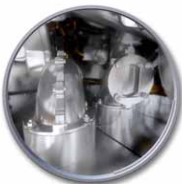
BUILT-IN NON RETURN SMOKE VALVES
